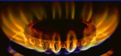
A ragged yellow/orange flame could mean carbon monoxide is present
